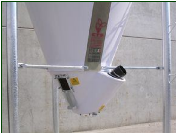
Code C8 Silos well. Unloading using a screw conv. at an inclination of 60^\circ D:780mm H:650mm
