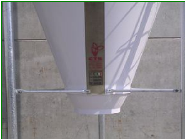
Code C2A Bottom reduction for automatic distribution system. D:780mm d:540mm H:230mm
