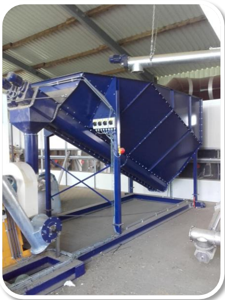
Oblique bunker 8m 3
