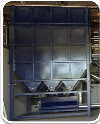
Intake bunker 48 m3
