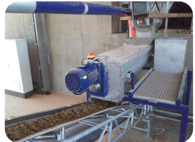
Mixed wet and dry manure on the conveyor belt to the Pollo dryer
