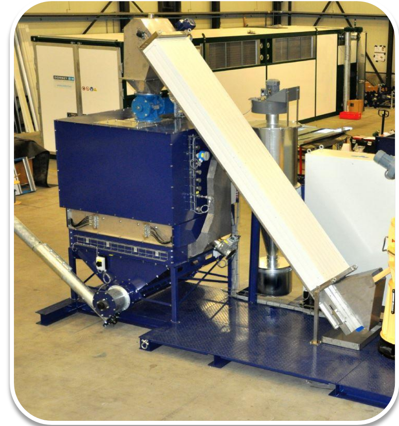
The Dorset sanitation unit consists of a rotary valve, the sanitation unit itself (including heating, high level sensor) and a pellet outlet at the bottom. Product is supplied to the sanitation by means of a heated belt.
