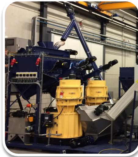
Pelletizing plant 800 kg/hour
