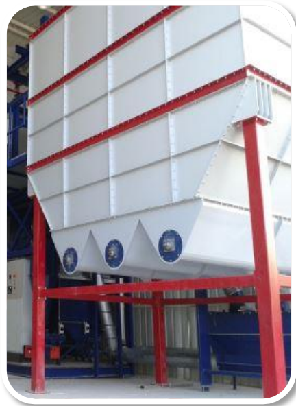
Steel intake bunker 27 - 54 m 3
