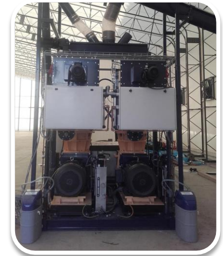
Pelletizing plant equipped with steam unit
